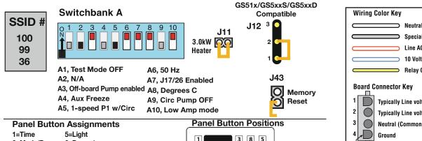
2=Mode/Prog 6=Pump 1 3=Temp Up 7=Pump 2 4=Temp Down 8=J17/26 1 3 8 5 2 4 6 7 Page 5
