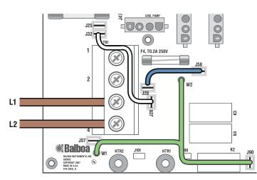
Single Service, IT Electrical System (No Neutral) Line - Line voltage is 230VAC (1 x 16 Amp or 1 x 32 Amp) 3 Wires (2 Lines + 1 Protective Earth)
