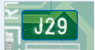
J29 is a heater disable switch input.
