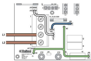
Single Service, IT Electrical System (No Neutral) Line - Line voltage is 230VAC (1 x 16 Amp or 1 x 32 Amp) 3 Wires (2 Lines + 1 Protective Earth)
